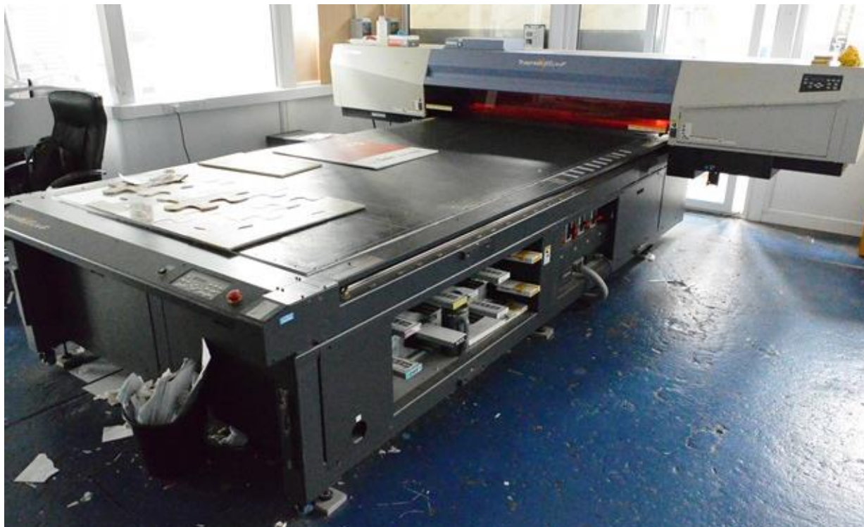
Screen Truepress Jet 1600 UVMF large format inkjet printer, 3100 x 1800mm (up to 50mm thick material), serial no. JFX-1631, 11405A160 (2010)
