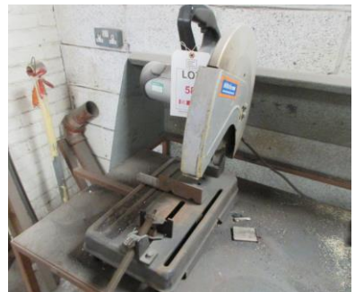
Evolution 500 bench top abrasive steel cutting saw
