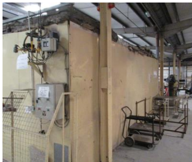
Unbadged gas fired walk-in sliding door drying room
