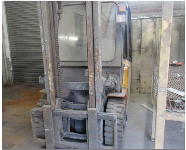
Heli HFB30 ride on duplex mast battery forklift
