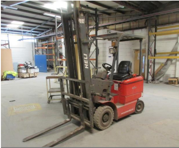
Heli HFB15 ride on duplex mast battery forklift
