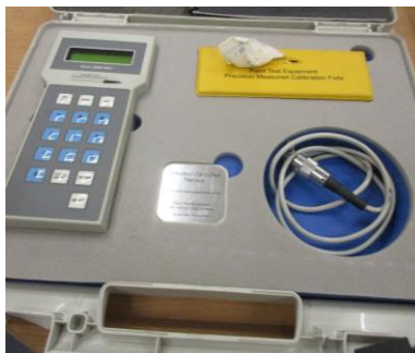
Eban 2000 MK2 hand held digital paint coating thickness meter
