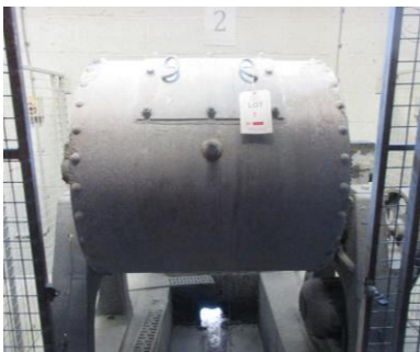
Barrel mixer / mill (50ff – ranging from 25-100kg)
