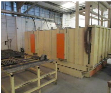
Unbadged front loading electric annealing furnace
