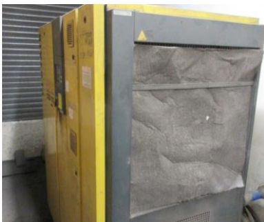
HPC Plusair rotary screw air compressor set, Type CSD102
